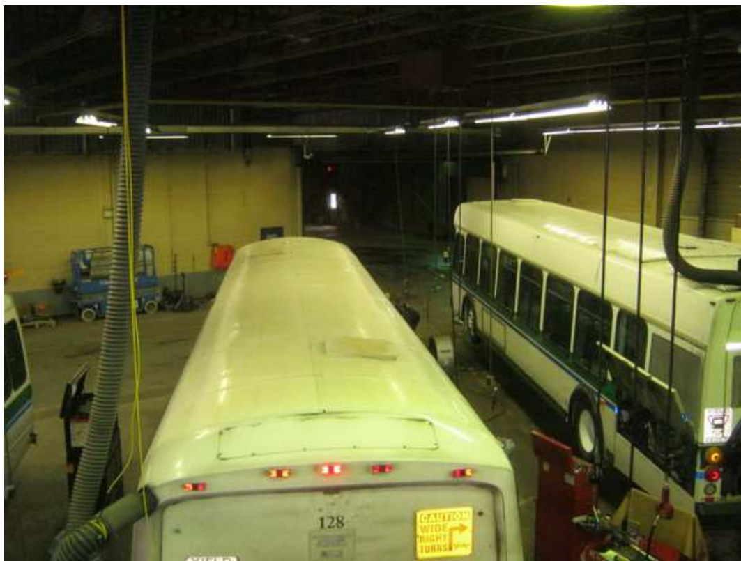
D309099 Maintenance Shop showing buses on hydraulic hoists
