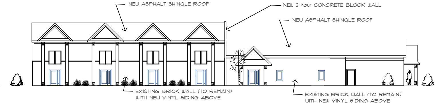
NORTH ELEVATION (LOOKING FROM RUTH ST) SCALE: NTS
