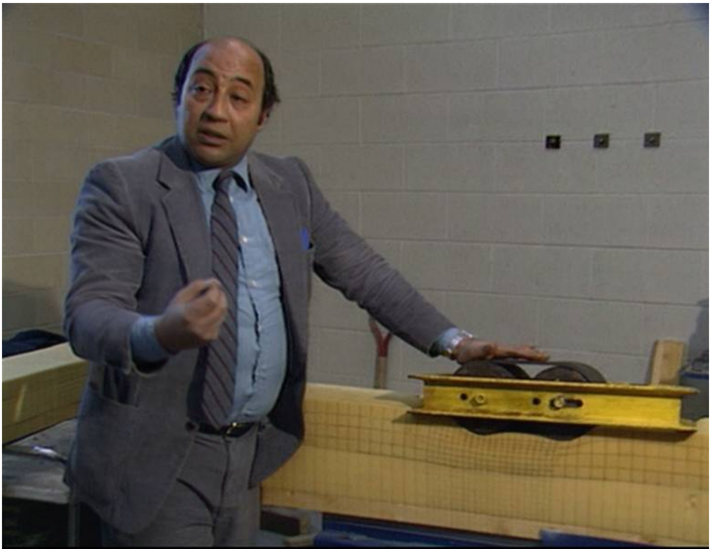
Abd El Halim demonstrates the concept behind his rubber-belted asphalt roller in 1987. (CBC)
