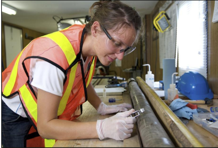
Researcher studies samples of limestone rock drilled from one of eight boreholes around DGR site.
